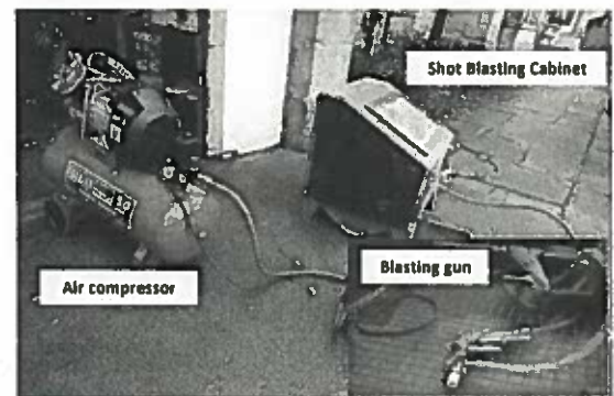
Fig. 2 The abrasive cleaning system.
