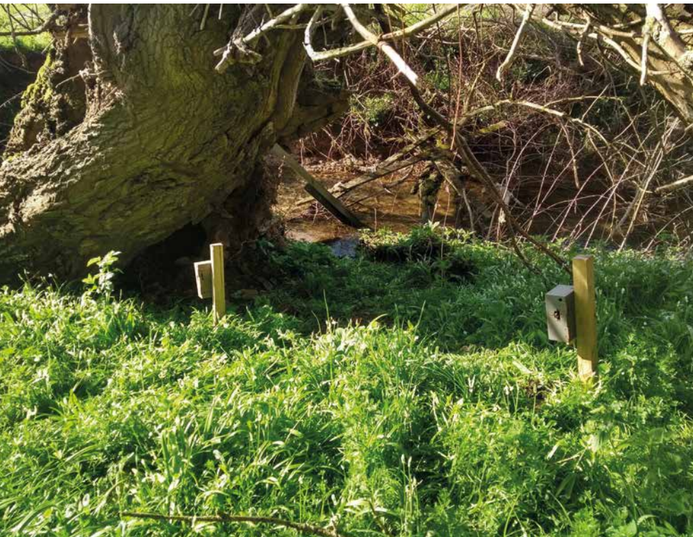
Figure 3. Example of camera-trap set-up at a potential resting or breeding site. Cameras are placed close to maximise detection probability while avoiding any obstruction to the entrance and run(s) and in pre-designed emplacements. This means that maintenance visits are quick because replacement camera traps with correct settings can be swapped quickly but maintain the same viewing angles. A view from the closer (left) camera can be seen in Figure 2.
