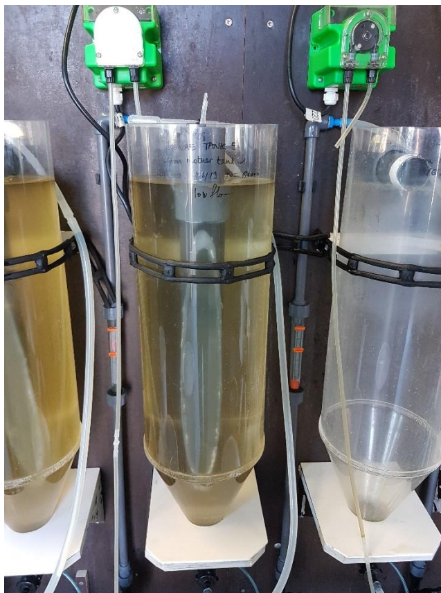
Figure 6.2 15L upwelling larval rearing tank on the flow-through system with continuous feed dosing system (green).
