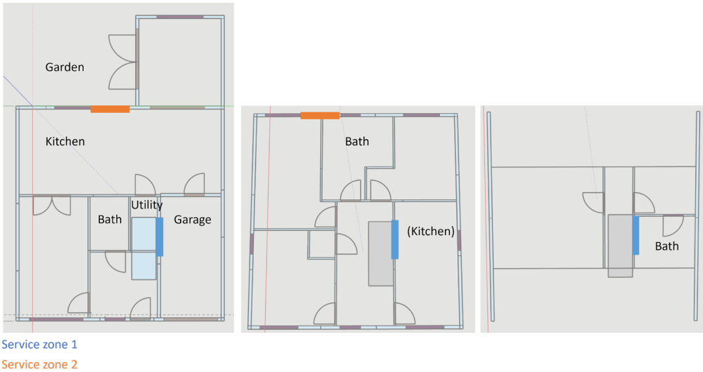
Figure 33 Service zones shown in the floor layouts of all floors. From left to right: Ground floor, first floor, second floor.
