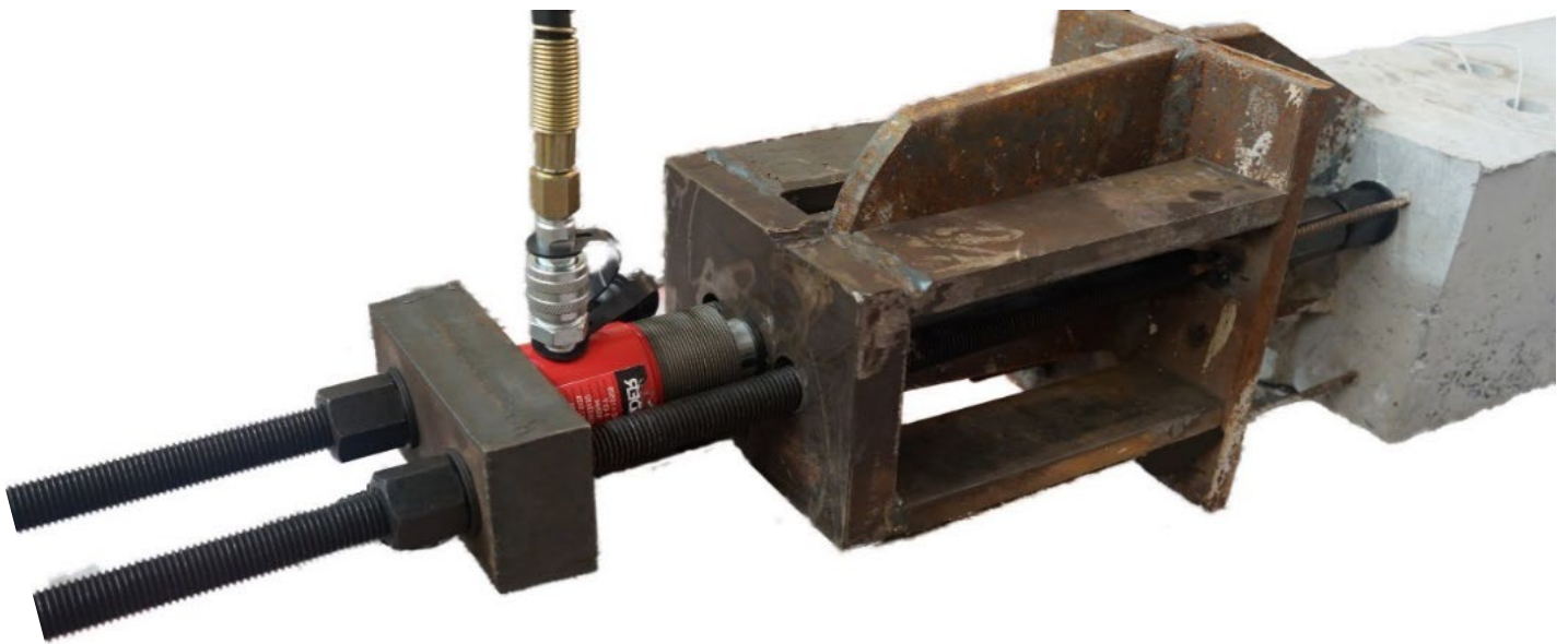
(b) Practicality picture of of the post-tension hydraulic device
