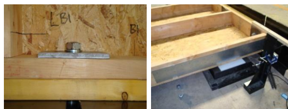
Figure 7: Method of securing the panel to the test rig (l) and detail restraint strap providing resistance to overturning forces (r).
