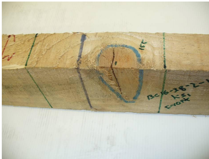
Figure 4-12 A spike knot is positioned in segment 3 of joist 05 of 2m joists
