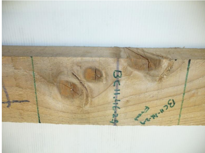
Figure 4-13 Three knots of 80% TKAR present in the 2.8m joist.
