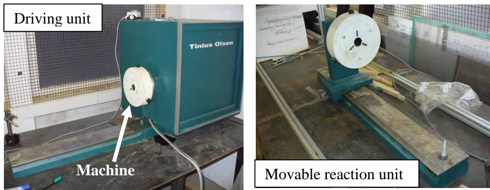
Figure 3-1 The driving house and the reaction bench of the torsion tester.
