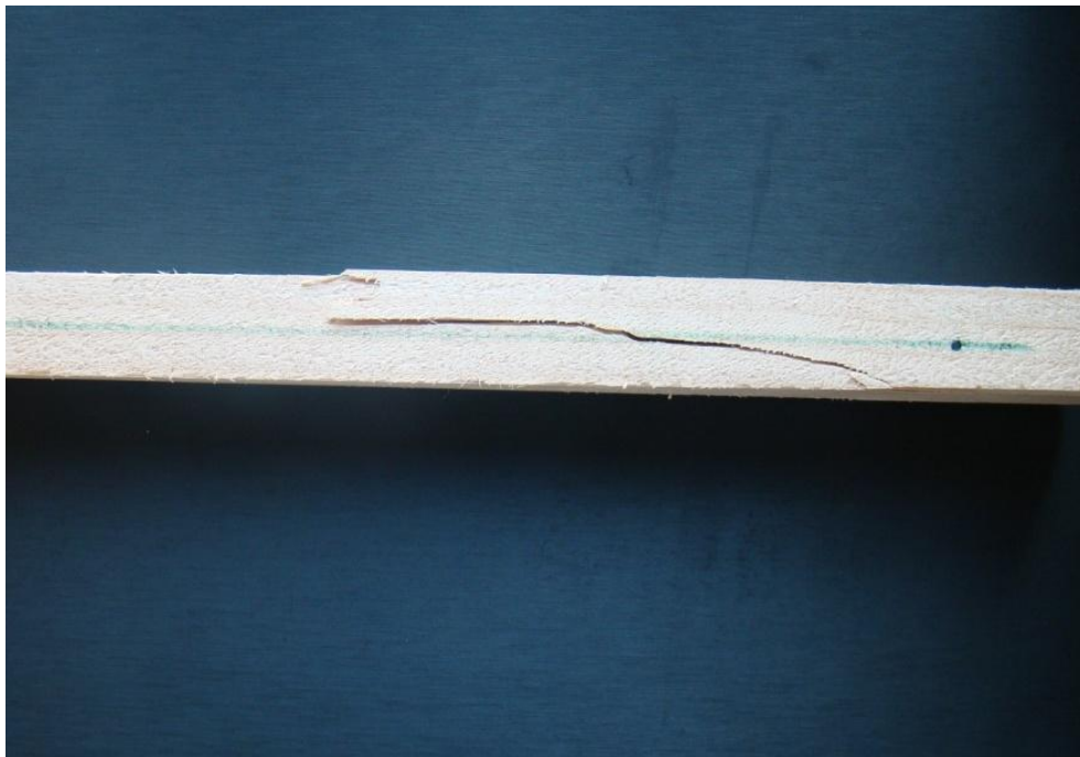
Figure 6-6 A typical shear failure occurred in clear wood specimen.
