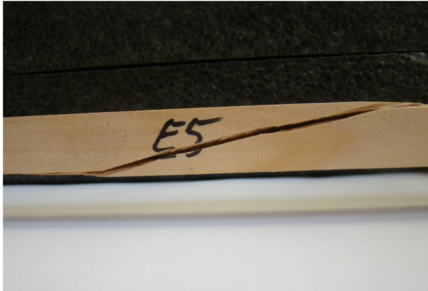
Figure 6-7 A typical combined shear tension failure occurred in clear wood specimen
