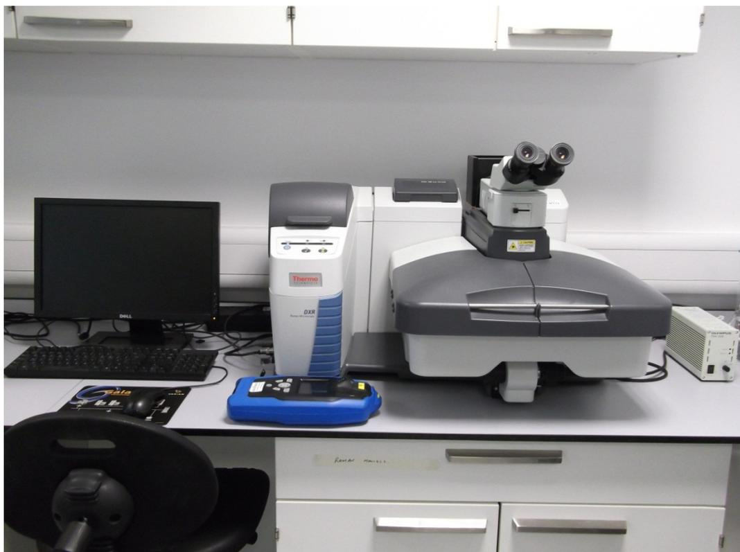
**Figure 3.8:** size comparison of DXR bench top Raman spectrometer and TruScan handheld Raman spectrometer
