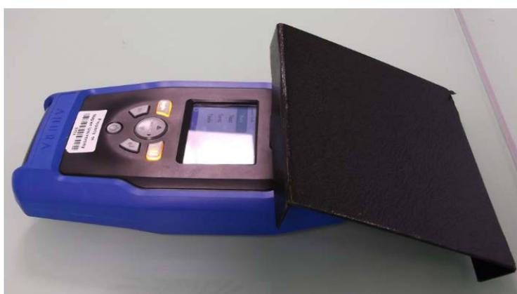
**Figure 5.2:** handheld Raman spectroscope covered with black opaque object
