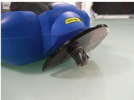
**Figure 3.7:** stone attached to the barrel-shaped nose cone for analysis using sellotape
