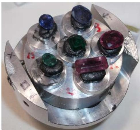
**Figure C1:** Two of each stone; rubies, sapphires and emeralds mounted on the chamber holder using a grey Plasticine® substance.
