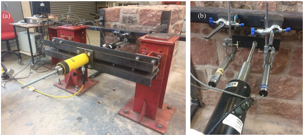
Fig. 5. (a) Overview of the experimental configuration for the pull-out test; (b) detail of the measuring equipment for anchor displacement (LVDTs).
