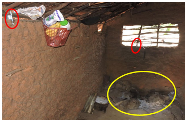
Figure 2. Sampling setup for CO passive diffusion tubes. Red circles indicate location of Dosi tubes, and the yellow circle shows the three-stone fire.
