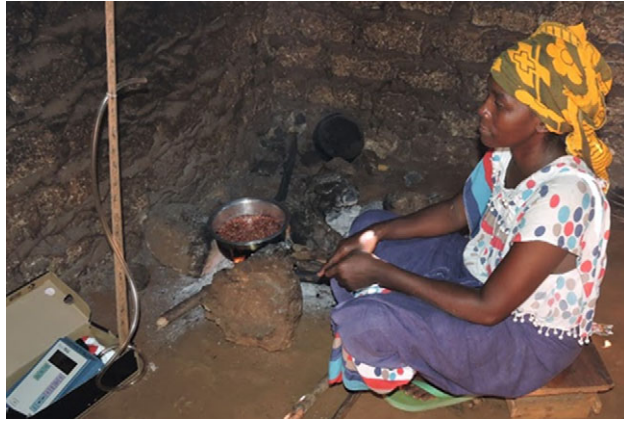
Figure 4. Sampling setup to measure particulate pollution during the cooking process in households.
