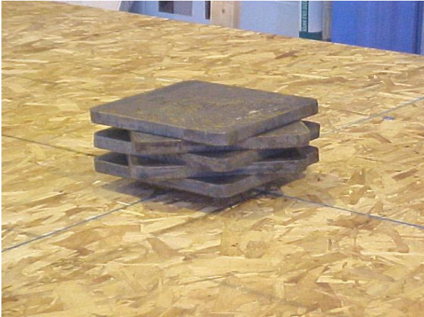
Figure 9: 1 kN load at centre of floor
