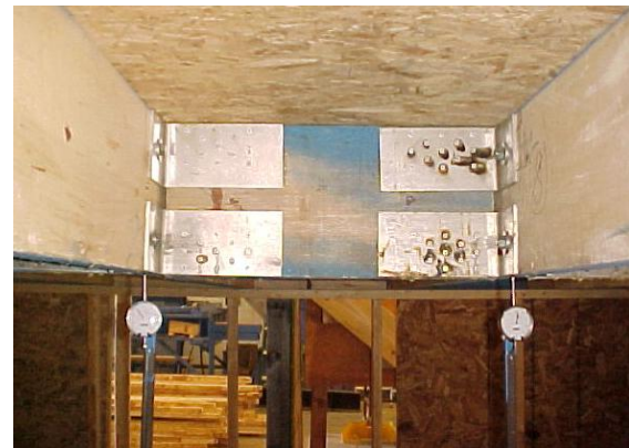
Figure 8: Artificial joist bracing method
